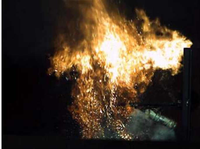
FIGURE 9. HIGH-SPEED VIDEO CAPTURE OF EXPLODING CELL.
