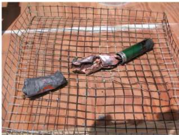
FIGURE 5. EXPLODED CELL AND ITS CONTENTS
